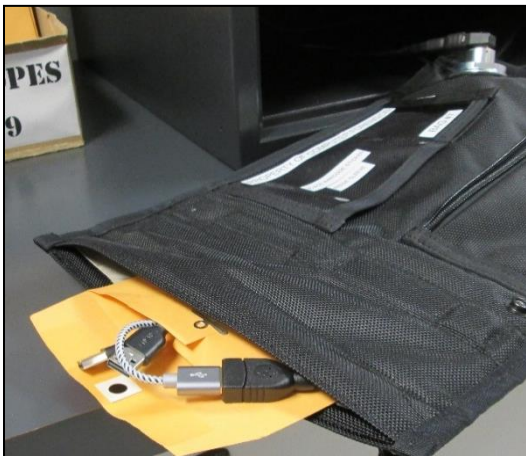
Connect power cable from inside of Faraday Bag to device charging cable
